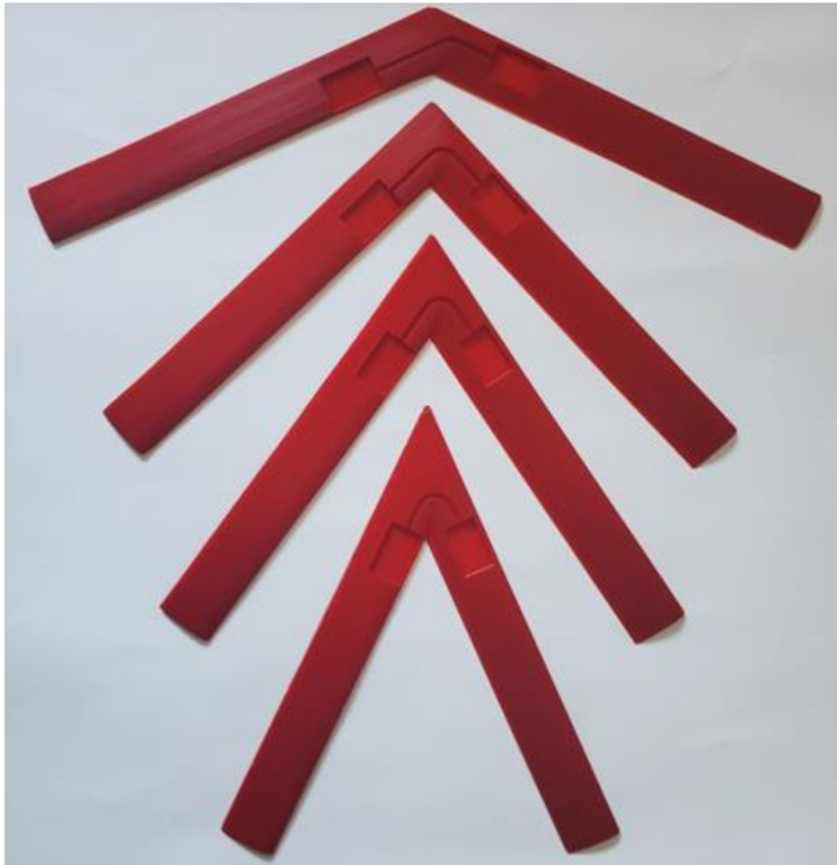
Fig. 4: Traditional-V 3D Printed Boomerangs with Varying Joint Angles
