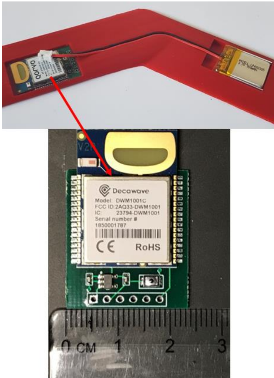
Fig. 5: Ultra-Compact Custom UWB Wireless Positioning Tag
