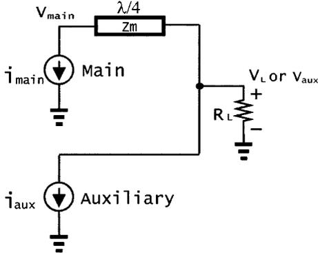
Fig. 3. Simplified output network used for analysis.
