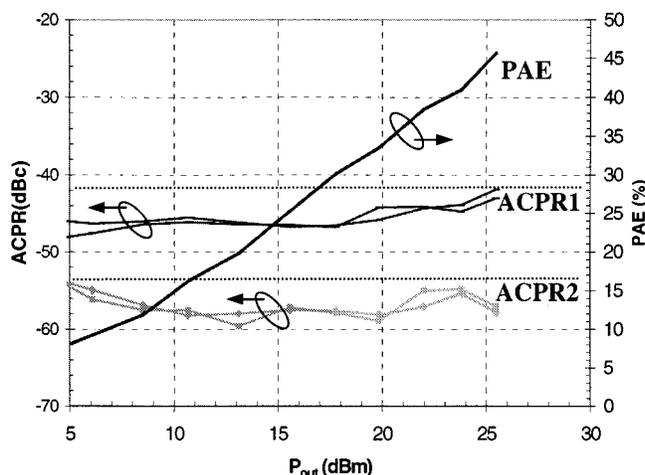
Fig. 12. Measured ACPR and PAE versus output power.
