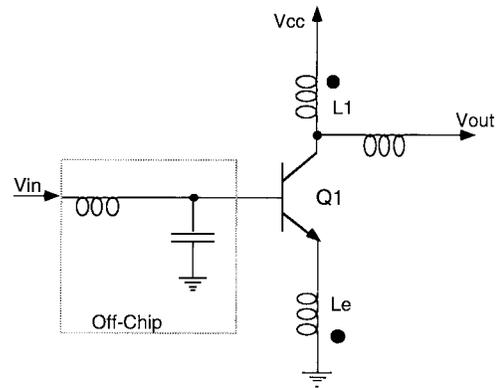
Fig. 7. Schematic of SiGe HBT low-noise amplifier with monolithic transformer coupling [24].
