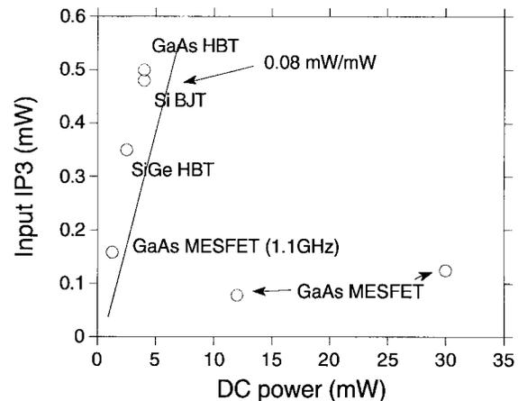
Fig. 5. Amplifier linearity figure-of-merit plotted for the same monolithic 2-GHz amplifiers of Fig. 4. The best results fall on a line of approximately 0.08 mW/mW [21]–[27].
