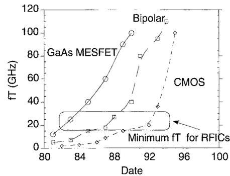
Fig. 3. Reported transistor cutoff frequency versus time [8]. Note that all silicon technologies are now capable of addressing applications in the 1–2 GHz regime.
