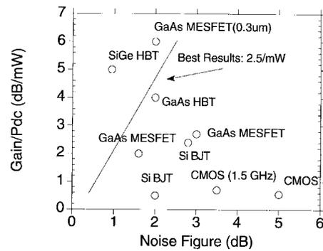
Fig. 4. Gain-to-dc power ratio plotted versus noise figure for state-of-the-art 2-GHz LNA's. The best results have a figure-of-merit of approximately 2.5/mW [21]–[27].
