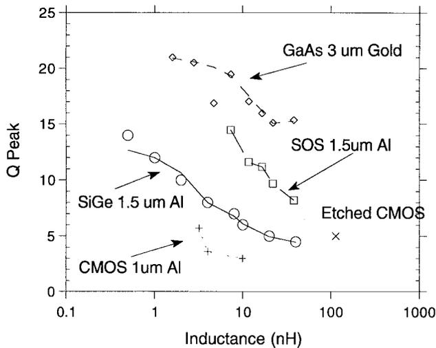
Fig. 12. Reported peak- $Q$  values of monolithic inductors as a function of inductance [56]–[59]. The highest values of peak inductor  $Q$  are obtained with semi-insulating substrates and relatively thick metallizations.
