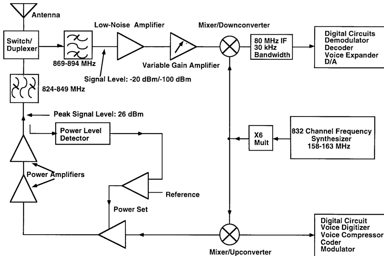
Fig. 1. Simplified block diagram of RF portion of IS-54/136 transceiver [2].
