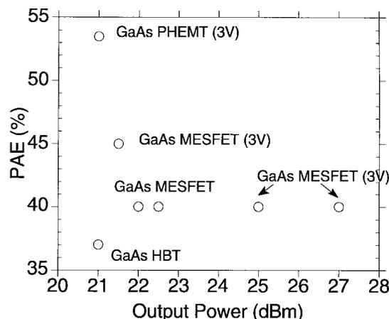
Fig. 9. PHS/PACS power amplifier performance for ACP  $< -55$  dBc at 600 kHz offset [75]–[80]. The best performance is obtained with a GaAs PHEMT.
