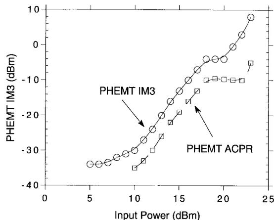
Fig. 8. Comparison of third-order IM power and adjacent-channel power for GaAs PHEMT [31]. Note that IM3 and ACPR track each other over a broad range of input power levels.
