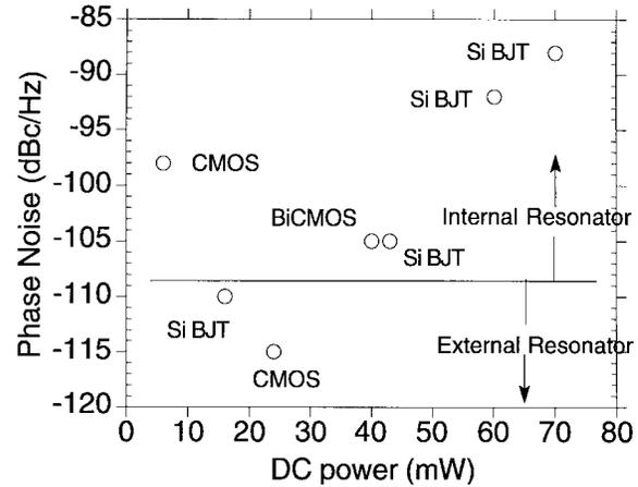
Fig. 10. Measured phase noise as a function of dc power for a variety of monolithic VCO circuits in the 2 GHz frequency range at an offset frequency of 100 kHz from the carrier [81]–[87]. The use of an external resonator provides the best noise performance.
