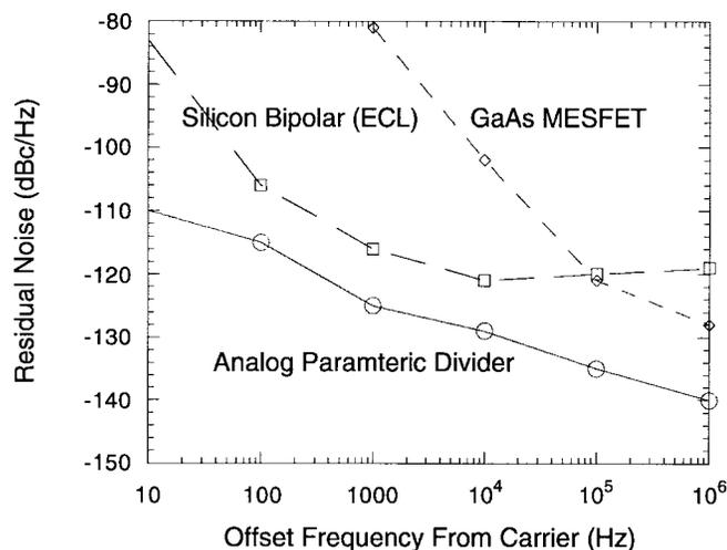
Fig. 11. Reported frequency divider residual phase noise normalized to 10 GHz [50]. Note that the lower phase noise of the silicon bipolar transistor results in lower residual divider phase noise.
