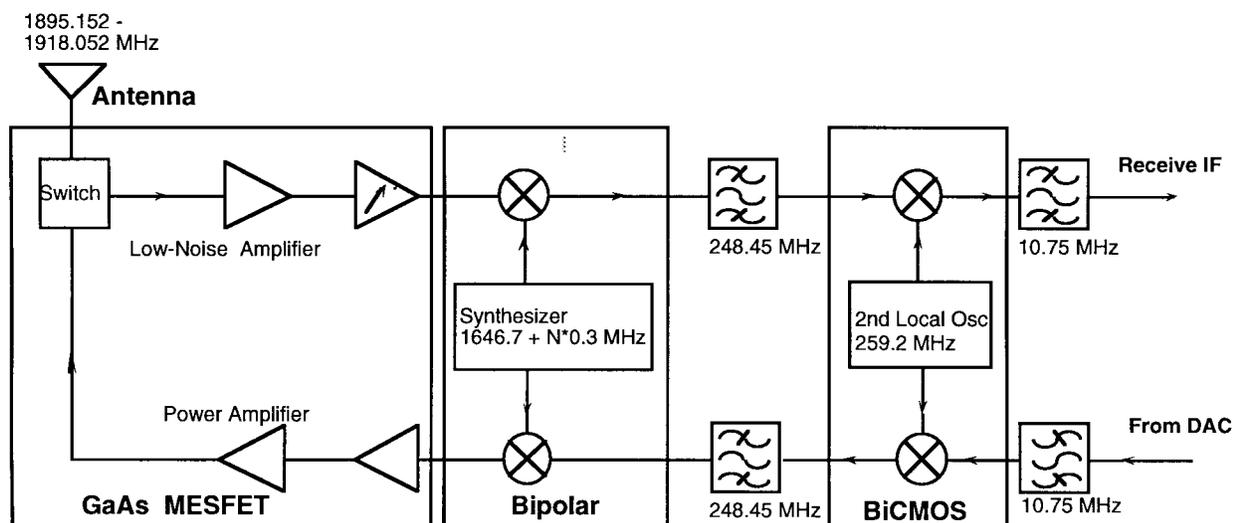
Fig. 2. Simplified block diagram of PHS transceiver [5].
