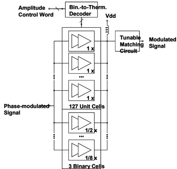
Fig. 6: Architecture of digital power amplifier based on control of number of unit cells.
