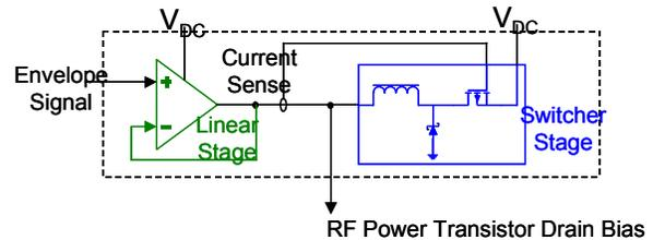
Fig. 4: Architecture of dynamic drain voltage supply for ET and EER amplifiers.
