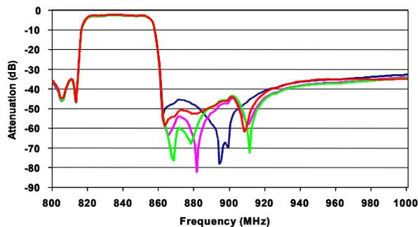
Fig. 8: Experimental transfer curves for duplexer enhanced with active feedforward noise cancellation [10]
