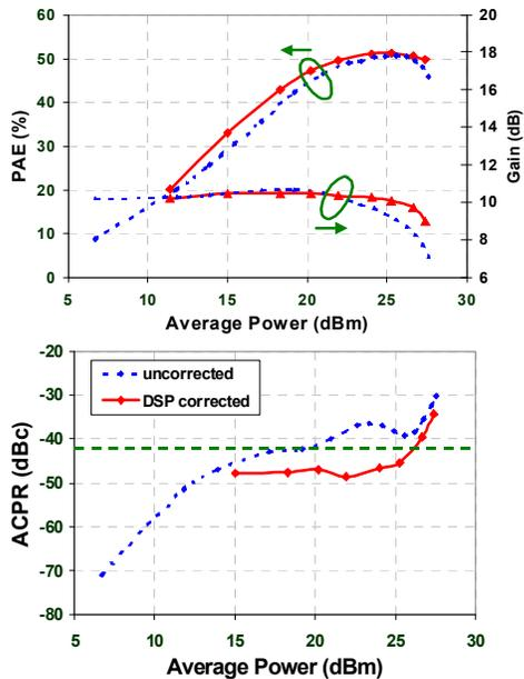
Fig.3: Experimental results for Doherty handset PA using CDMA inputs. Results before and after digital predistortion are shown.
