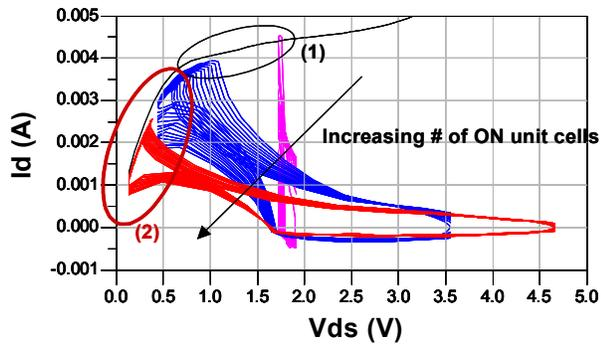
Fig. 7: Simulated variation of load lines in digitally controlled PA as output power changes.
