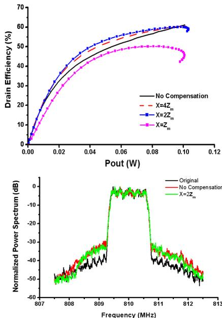
Fig. 5: Experimental results for CMOS amplifier with Chireix combiner: a) efficiency for CW signals; b) spectrum with CDMA signal.
