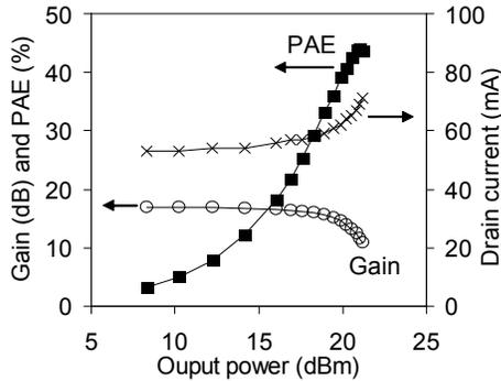
Fig.2: Experimental results for 3 stacked nMOS amplifier using SOS technology.
