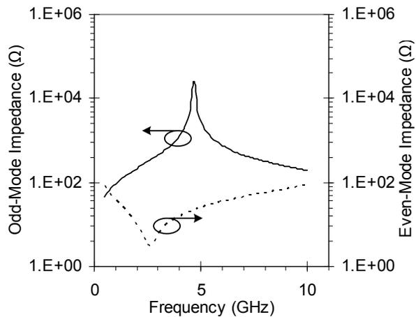
Fig. 6 Simulated performance of coupled inductor transformer.
