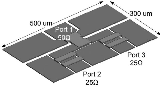
Fig. 4 3D layout of the wideband output balun.
