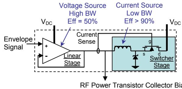
Figure 4: Schematic diagram of high efficiency envelope amplifier.
