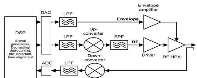
Figure. 1. Block diagram of envelope tracking base-station amplifier
