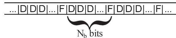
Fig. 1. Binary block code that is showing a block of N_b bits with the flag bit F denoting the polarity of the associated block of bits.
