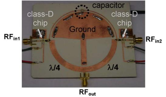
Fig. 4. Photograph of the CMOS outphasing Class-D PA with the Chireix combiner realized by a half wave length transmission line.
