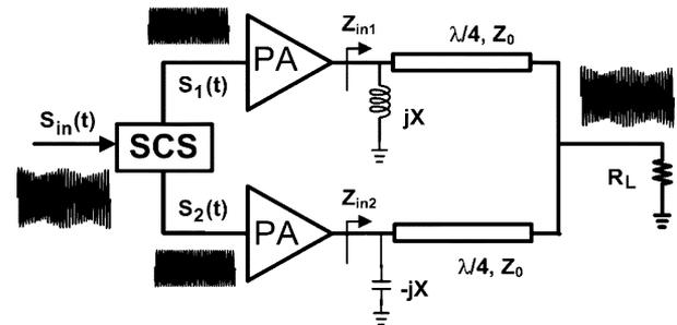
Fig. 1. Simplified block diagram of an outphasing system with a Chireix combiner. The compensation reactances are complex conjugate ( $\pm jX$ ).
