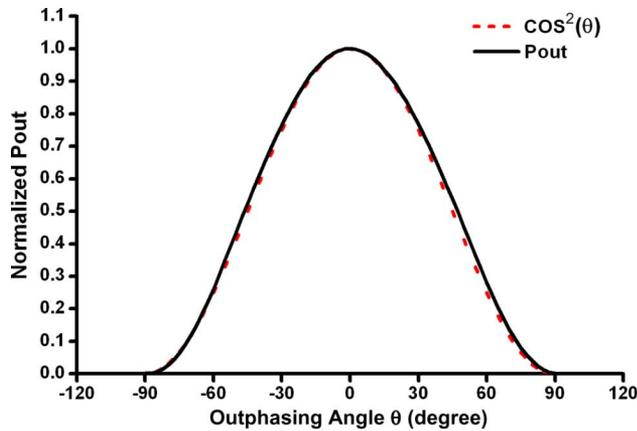
Fig. 6. Normalized measured output power versus outphasing angle  $\theta$ . A  $\cos^2 \theta$  curve is shown for comparison.
