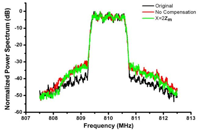
Fig. 8. Measured PA output spectrum with CDMA signals. An ACPR of  $-45$  dBc was achieved.
