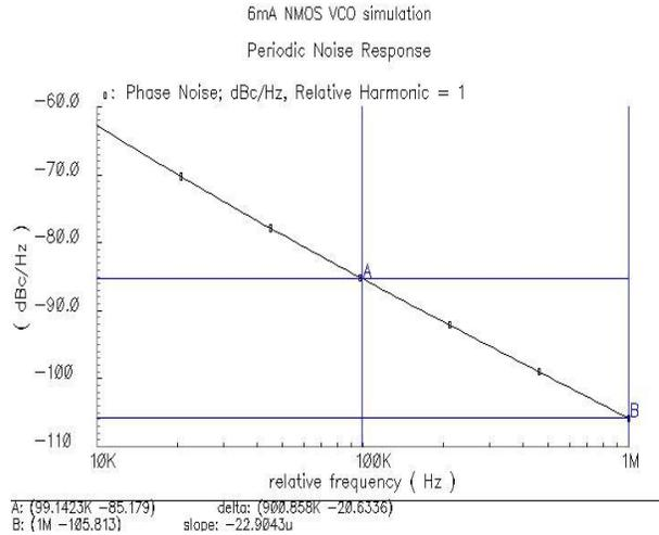
Fig. 6. Simulated plot of VCO Phase Noise
