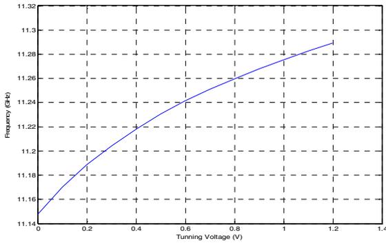
Fig. 3. Measured VCO tuning at 11.2GHz
