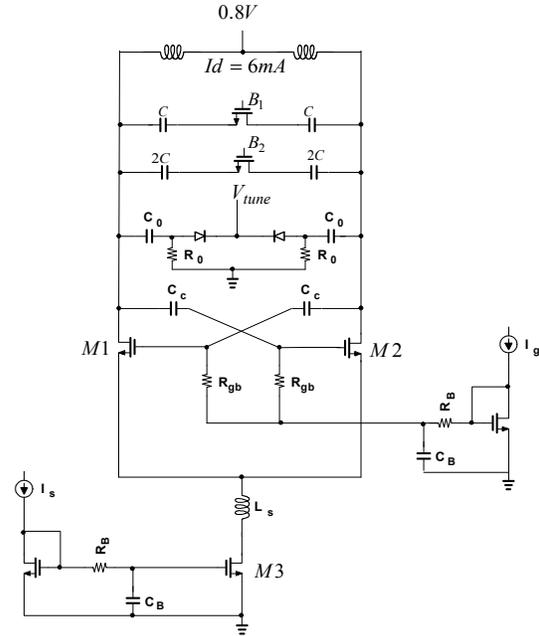
Fig. 1. VCO Schematic
