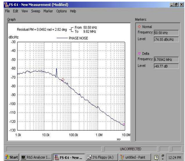
Fig. 7. Measured phase noise at 11.2GHz
