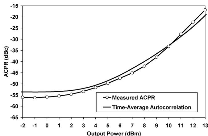
Fig. 10. Measured and calculated ACPR for CDMA reverse-link signal.
