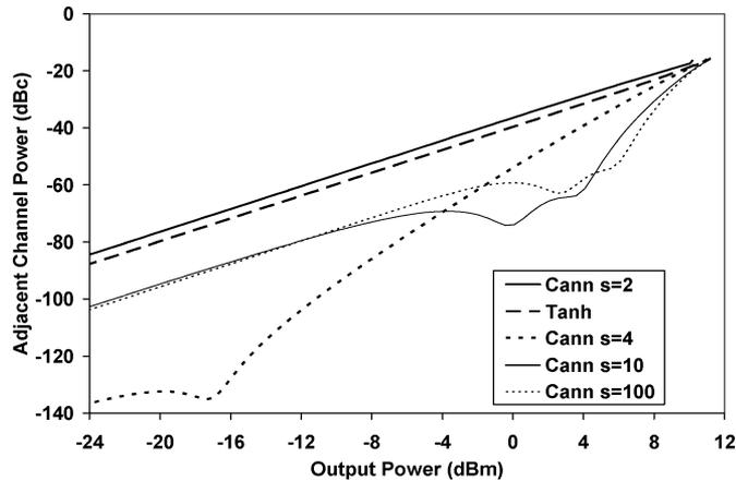
Fig. 6. Adjacent channel power at 885-kHz offset for limiter models.
