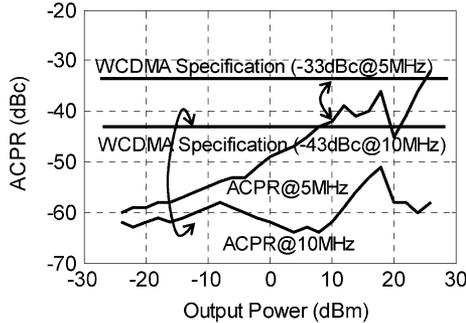
Fig. 20. Measured ACPRs of DCB SiGe HBT PA.
