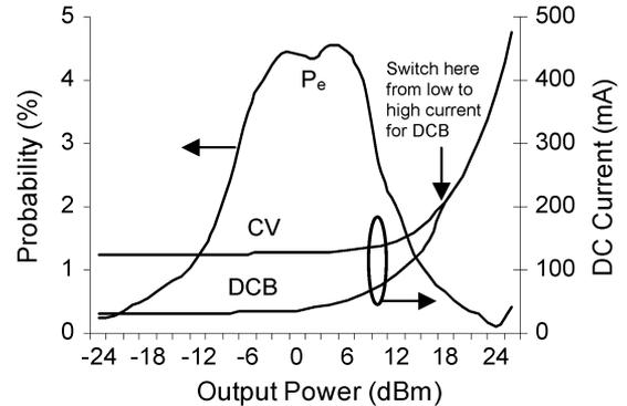
Fig. 17. Output power probability distribution  $P_e$  and measured dc current for different biasing techniques. The switch point from 100 devices to 20 devices occurs at  $P_{\text{out}} = 18 \text{ dBm}$ .  $V_{CC} = 3 \text{ V}$ .
