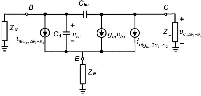
Fig. 21. Equivalent circuit for the computation of the third-order intermodulation product  $2\omega_1 - \omega_2$ .
