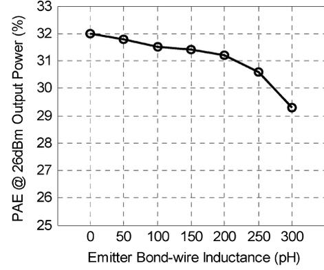
Fig. 9. Simulated PAEs at 26-dBm output power with different values of  $L_e$ .
