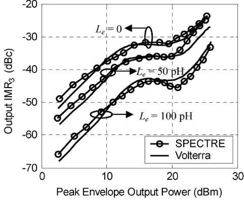
Fig. 7.  $\text{IMR}_3$  with different values of  $L_e$ ,  $I_{CQ} = 110$  mA.
