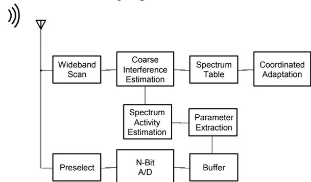
Fig. 1: General system architecture of “cognitive radio” [8].
