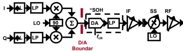
Fig. 3: Digital IF transmitter architecture from [14]. In this case, I/Q modulation of the IF is performed in the digital domain. This places a greater burden on the DAC than traditional approaches, though improved DAC architectures can minimize this limitation.
