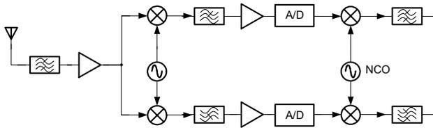
Fig. 2: Digital IF receiver architecture. In this case, the final stage of downconversion and image rejection is done in the digital domain. This places a greater burden on the ADC than more traditional approaches.
