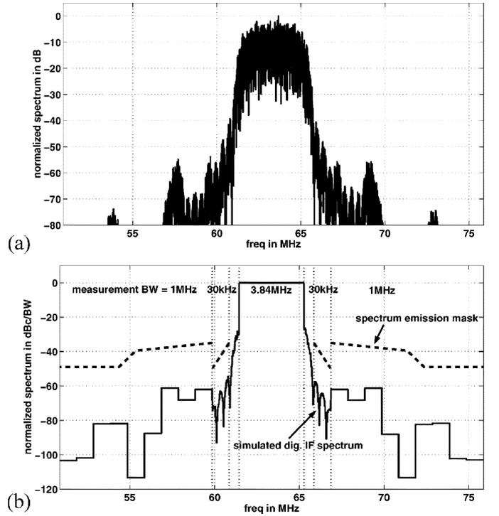
Fig. 13. (a) Spectrum of the digital-IF signal and (b) the corresponding spectrum expressed in dBc over the respective measurement bandwidth.
