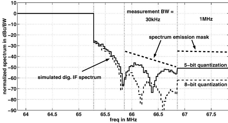
Fig. 14. Spectrum of the digital-IF signal in dBc over measurement bandwidth with 5 or 8 bit of resolution.
