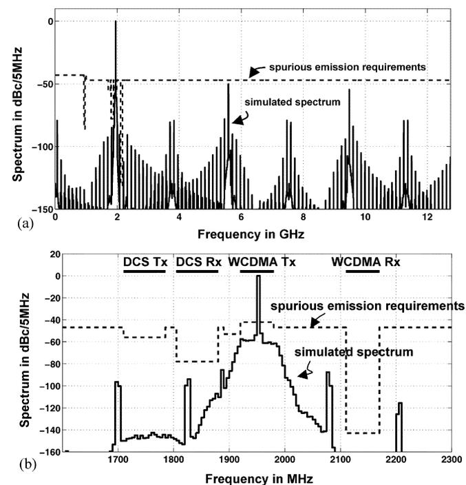
Fig. 20. Transmit signal spectrum at the antenna, expressed in dBc/5 MHz, (a) from DC to 12.5 GHz and (b) near the DCS/W-CDMA bands. Maximum (worst case) TxIC output power of 24 dBm is assumed.
