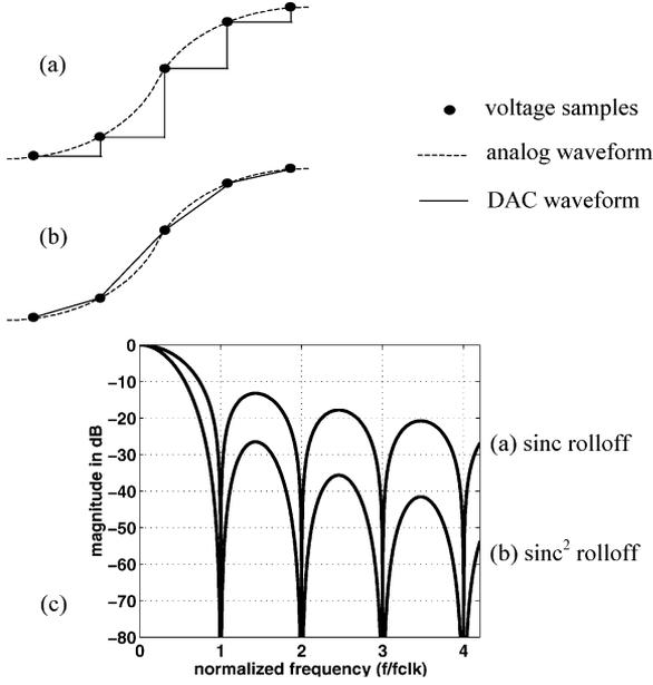
Fig. 7. Transient waveforms of (a) S/H DAC, (b) FOH DAC, and (c) their corresponding spectrum rolloffs.
