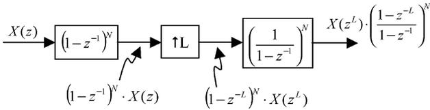
Fig. 12. Efficient implementation of a  $N$ -th-order comb low-pass filter for an  $L$ -times interpolation.
