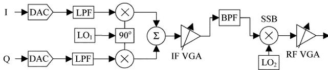
Fig. 1. Block diagram of a conventional heterodyne transmitter.
