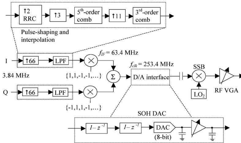
Fig. 15. Proposed transmitter architecture featuring a SOH DAC.
