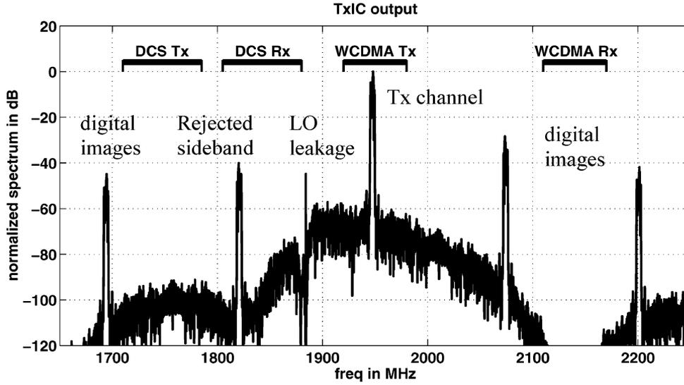
Fig. 17. Simulated output spectrum of the TxIC in the DCS and W-CDMA bands.
