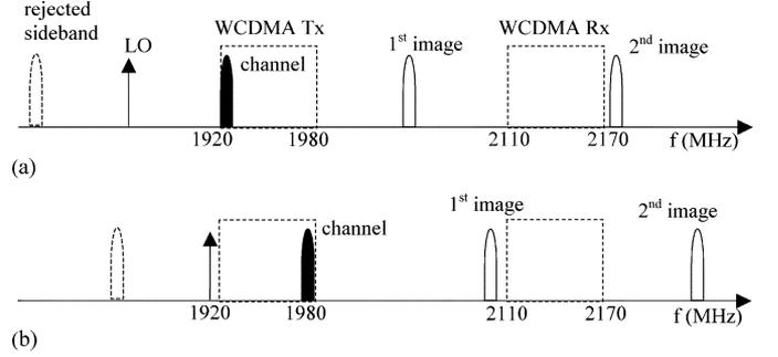
Fig. 6. Frequency planning: locations of images when the channel is at (a) the lower or (b) upper edge of the W-CDMA Tx band.
