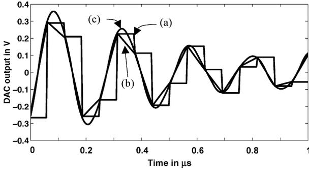
Fig. 9. Output waveforms of the (a) ZOH, (b) FOH, and (c) SOH DAC.
