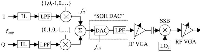
Fig. 4. Heterodyne transmitter with digital IF modulator.
