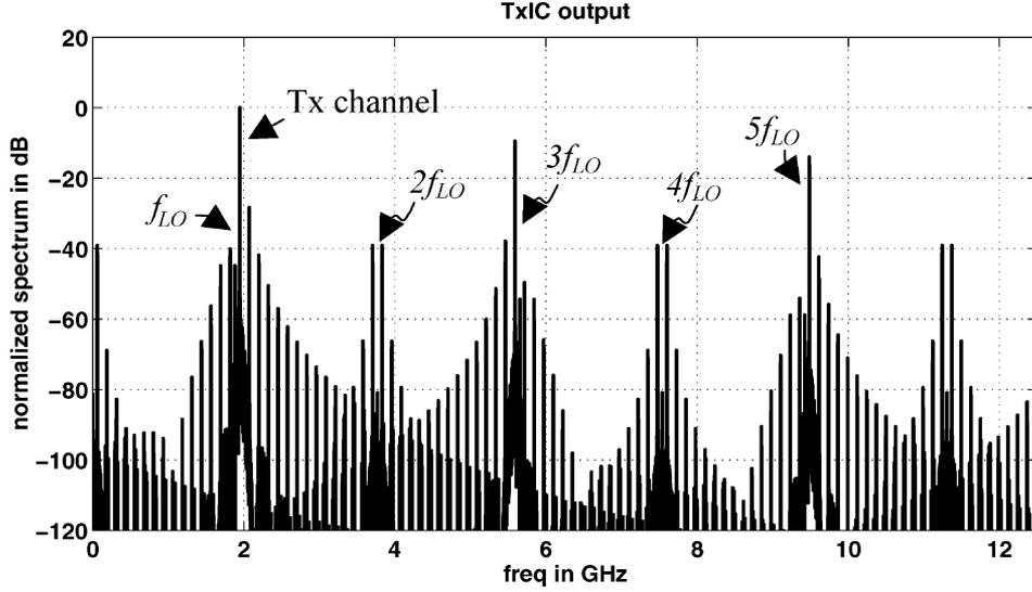
Fig. 16. Output spectrum of the TxIC from dc to 12.5 GHz.
