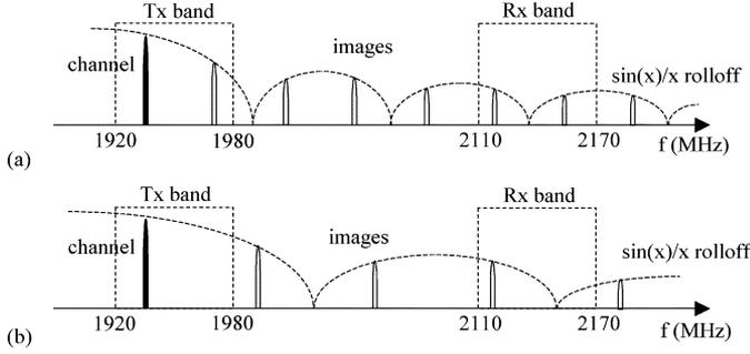
Fig. 5. Locations of digital images when (a)  $L = 16$ , and (b)  $L = 32$ . The “black” signal is the desired signal and the “white” are the digital images.
