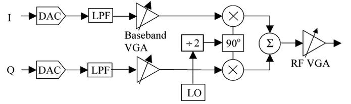
Fig. 3. Block diagram of a typical homodyne transmitter.
