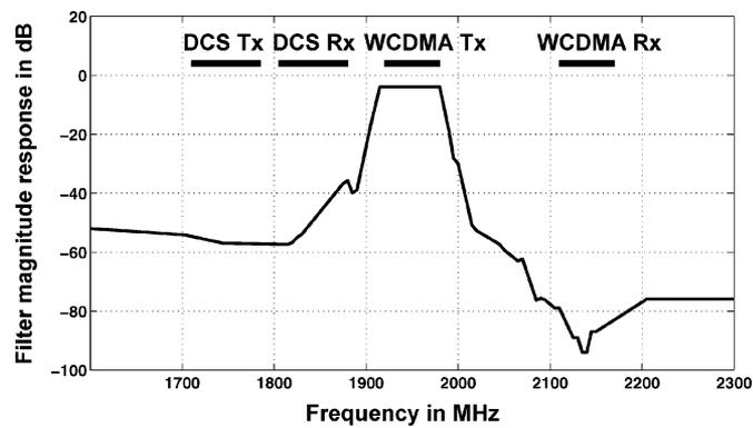
Fig. 19. Combined magnitude responses of the RF bandpass SAW filter and the duplexer filter.
