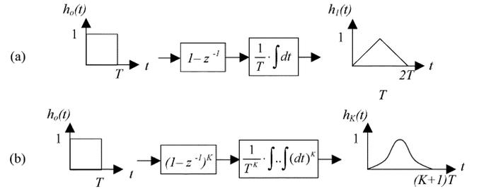
Fig. 8. Signal processing of (a) a FOH DAC and (b) a  $K$ th-order hold DAC.
