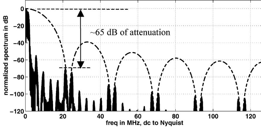
Fig. 11. Spectrum of the  $11 \times$  upsampled signal after the third-order comb filter ( $f_{\text{clk}} = 253.44$  MHz).
