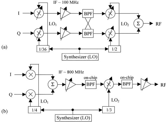
Fig. 2. Two variable-IF heterodyne architectures that eliminate the external IF filter by (a) implementing a complex-IF filter and (b) adopting a frequency-planning scheme.
