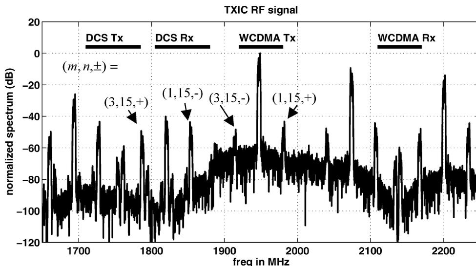
Fig. 18. Simulated output spectrum of the TxIC when the SOH DAC is replaced by a conventional ZOH DAC.
