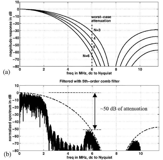
Fig. 10. (a) Magnitude responses of the comb filter of order 3–6 and (b) the filtered  $3 \times$  upsampled spectrum ( $f_{\text{clk}} = 23.04$  MHz).
