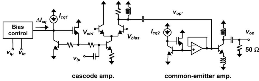
Fig. 15. Simplified schematic of the RFVGA. The two-stage design features adaptive bias schemes to make linearity requirements while minimizing the quiescent current consumptions.
