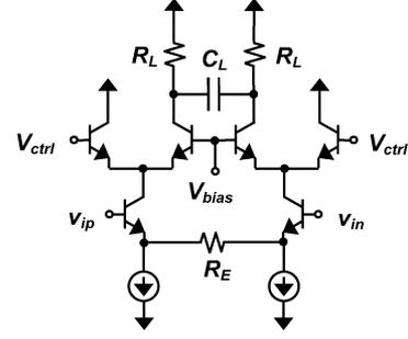
Fig. 10. Schematic of the IFVGA. It implements the second integrator for the SOH D/A conversion.
