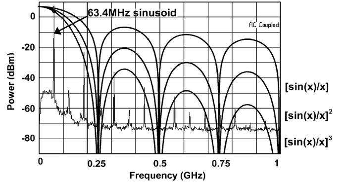
Fig. 11. Measured SOH DAC output spectrum from dc to 1 GHz. It exhibits the elevated  $[\sin(x)/x]^3$  image roll-off.
