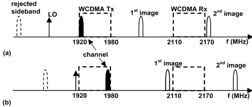
Fig. 4. Frequency planning illustration: locations of images when the channel is at (a) the lower or (b) the upper edge of the WCDMA Tx band. Images will always skip the forbidden Tx and Rx bands, thus substantially relaxing the filter requirements.
