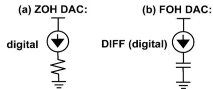
Fig. 6. Conceptual implementations of (a) the (conventional) current-steering ZOH DAC and (b) the FOH DAC. They are very comparable.
