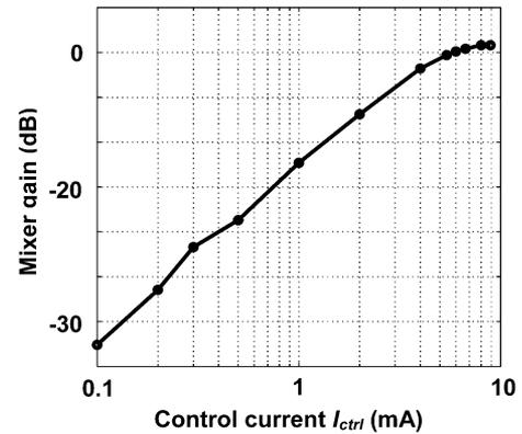
Fig. 14. Measured mixer gain versus the control current ( $I_{ctrl}$ ).
