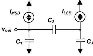
Fig. 9. Single-ended conceptual diagram of the 16-to-1 capacitor divider network.
