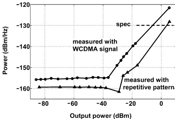
Fig. 24. Measured TxIC noise in the WCDMA Rx band.
