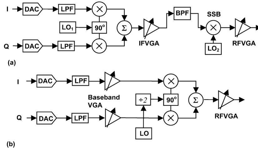
Fig. 2. Conceptual block diagrams of (a) the heterodyne and (b) the homodyne transmitter architecture.
