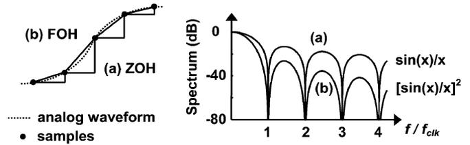
Fig. 5. Transient waveforms of (a) the ZOH (S/H) DAC and (b) the FOH DAC and their corresponding spectrum rolloffs.
