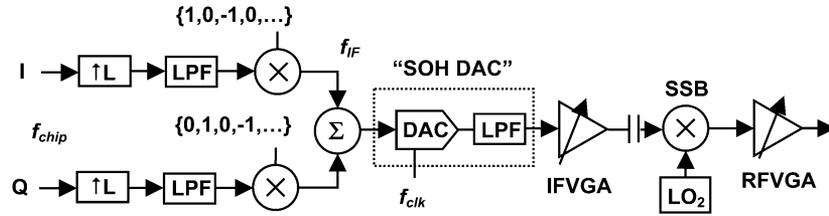
Fig. 3. Conceptual block diagram of the digital-IF heterodyne transmitter.
