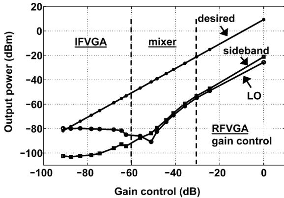
Fig. 22. Measured TxIC residual sideband and LO leakage.
