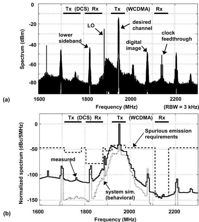
Fig. 21. (a) The measured TxIC output spectrum in the DCS and WCDMA bands (resolution bandwidth equals 3 kHz). (b) Normalized and including the external filter attenuation, it is shown to meet the spurious emission requirements.
