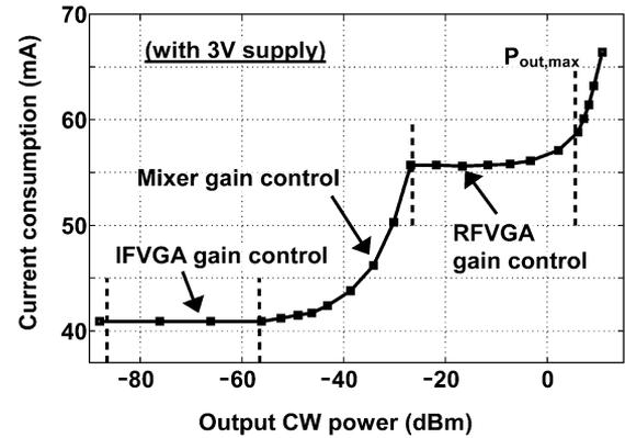
Fig. 25. Measured TxIC current consumption. It exhibits substantial power savings for power backoff mode.
