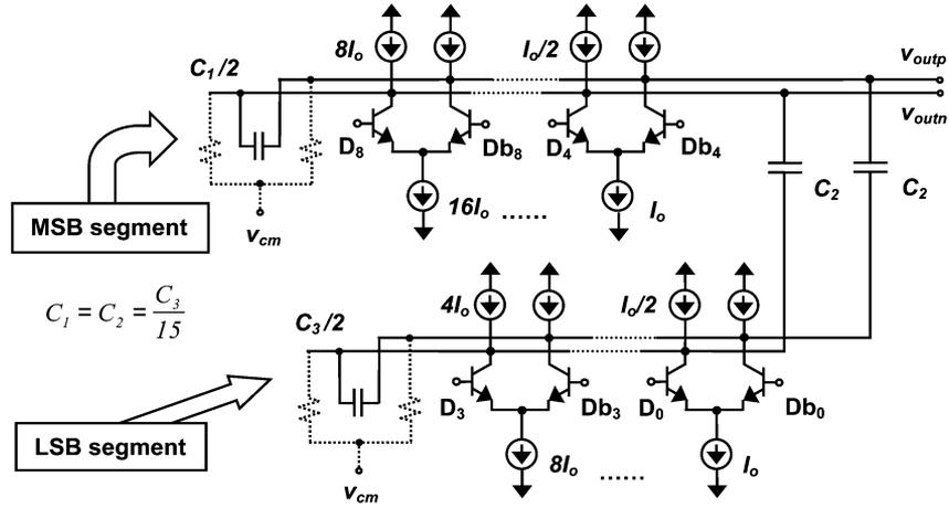
Fig. 8. Simplified schematic of the SOH DAC core, featuring the dominantly capacitive load.
