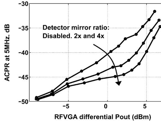
Fig. 19. Measured RFVGA ACPR results versus output power. Linearity improvement is observed over a wide range of power level.
