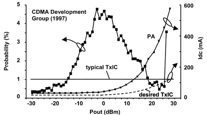
Fig. 1. Current consumption of PA and TxIC versus the transmitter output power, and the output power probability distribution function. A poorly designed TxIC can substantially reduce overall transmitter efficiency.
