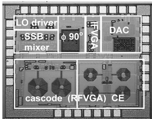
Fig. 20. TxIC chip microphotograph. It measures  $1.8 \times 2.2 \text{ mm}^2$ .
