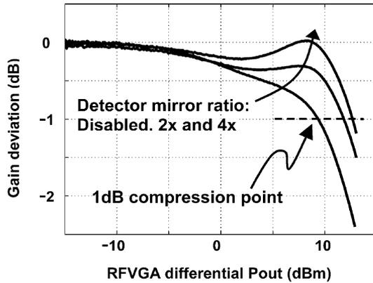
Fig. 17. Measured gain compression of the RFVGA versus output power level. Due to the current boost, gain compression is compensated for by gain expansion, thus increasing the 1-dB compression point by 3.5 dB.
