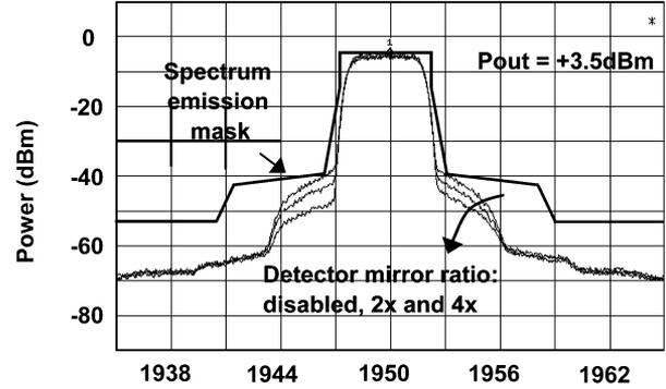
Fig. 18. Measured ACPR of RFVGA showing the linearity improvements due to the power-detector bias control.
