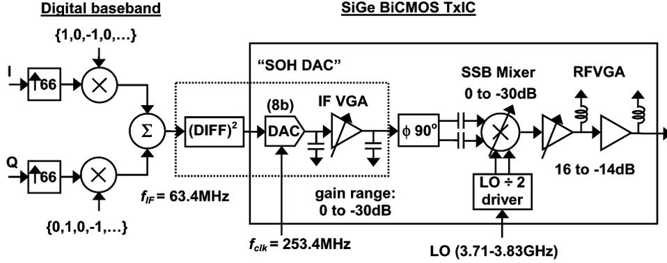
Fig. 7. Proposed digital-IF TxIC architecture. Employing the optimized frequency plan and the SOH DAC, spurious emission requirements are met with no dedicated IF filters.
