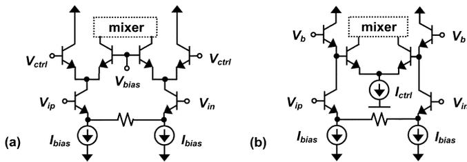
Fig. 13. Implementation of mixer variable-gain through (a) a bleeder circuit and (b) a translinear stage. The translinear circuit is more power-efficient as current consumption will drop with the mixer gain simultaneously.
