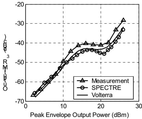
Fig. 5.  $IMR_3$  comparison between SPECTRE simulation, Volterra calculation, and measurement for the circuit of Fig. 4.
