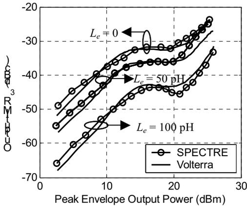
Fig. 7. IMR<sub>3</sub> with different values of  $L_e$ ,  $I_{CQ} = 110$  mA.
