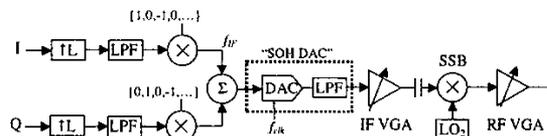
Figure 2. Heterodyne transmitter with digital IF modulator
