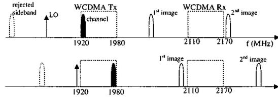
Figure 4. Frequency planning illustration: locations of images when the channel is at the lower or the upper edge of the Tx band.
