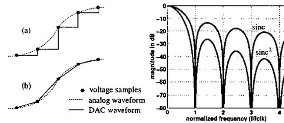
Figure 5. Transient waveforms of (a) S/H DAC and (b) FOH DAC, and their corresponding spectrum rolloffs.
