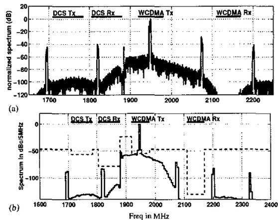
Figure 9. Spectrums, (a) at the output of the transmitter, and (b) at the antenna (after being filtered by the RF SAW and the duplexer).
