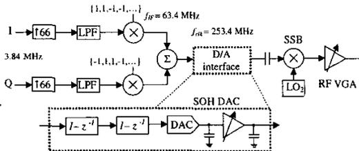
Figure 8. The proposed transmitter architecture which features a SOH DAC.
