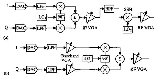
Figure 1. Block diagrams of (a) the heterodyne, and (b) the homodyne transmitter architecture
