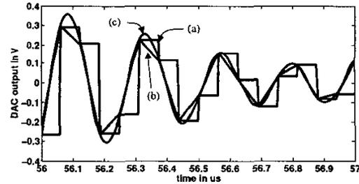
Figure 7. Output waveforms of the (a) ZOH, (b) FOH, and (c) SOH DAC
