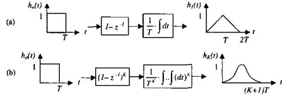
Figure 6. Signal processing of (a) a FOH DAC and (b) a  $K^{\text{th}}$ -order hold DAC.
