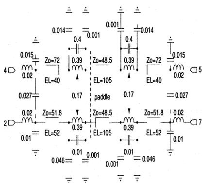
Fig. 7. Prototype ECPWFG package equivalent circuit. Capacitance, and inductance is in pF and nH, respectively. Electrical length (EL) is at 10 GHz, and  $Z_o$  is characteristic impedance in  $\Omega$ . Wirebonds have  $0.2 \Omega$  series resistance (not shown).
