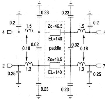
Fig. 3. SSOP8 equivalent circuit. Capacitance, and inductance is in pF and nH, respectively. Electrical length (EL) is at 10 GHz, and  $Z_o$  is characteristic impedance in  $\Omega$ . Series inductances have  $0.25 \Omega$  series resistance (not shown).
