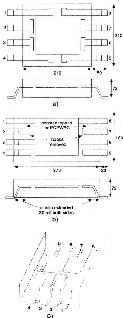
Fig. 1. Package structures: (a) traditional SSOP8; (b) proposed modified SSOP8 (ECPWFG package). Lead pitch is varied in the modified case to present  $50 \Omega$ , and packages are simulated with microstrip line Thrus as shown in the 3-D view of the modified package (c).
