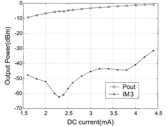
Fig. 12. Measured third-order intermodulation versus dc-bias current.  $P_{in} = -22$  dBm.
