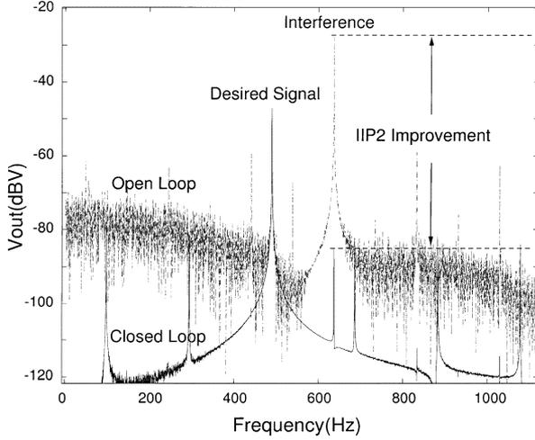
Fig. 9. Simulated closed-loop second-order nonlinearity cancellation result.
