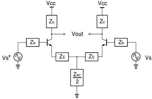
Fig. 2. Large-signal model of a CE differential pair.
