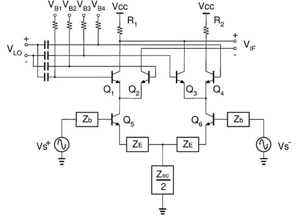
Fig. 3. Simplified model of bipolar double-balanced mixer.
