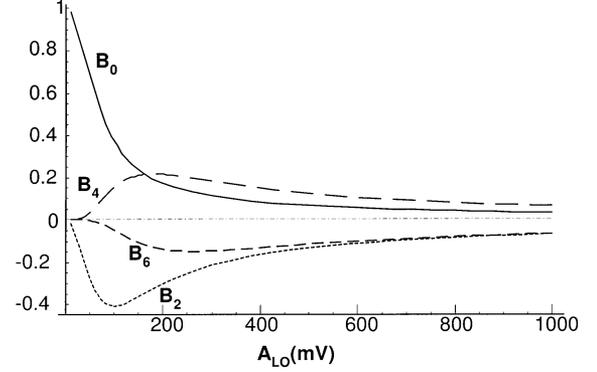
Fig. 4. Fourier-transform coefficients of the mismatch transfer function  $\operatorname{sech}^2(V_{LO}/2V_T)$ .  $B_0$  is the primary component affecting IIP<sub>2</sub>.
