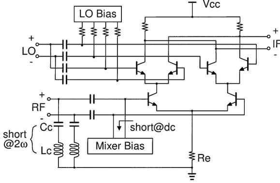
Fig. 5. Down-conversion double-balanced active mixer with third-order cancellation.
